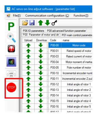
After successfully changing the parameter and confirming with Enter, this individual parameter (or all parameters) must be transferred to the motor driver via the green down arrow ( ). The power supply must not be interrupted during transfer. At the start of the data transfer, a pop-up window appears with a status bar for the transfer. After successful transfer, this is displayed under the status bar.
